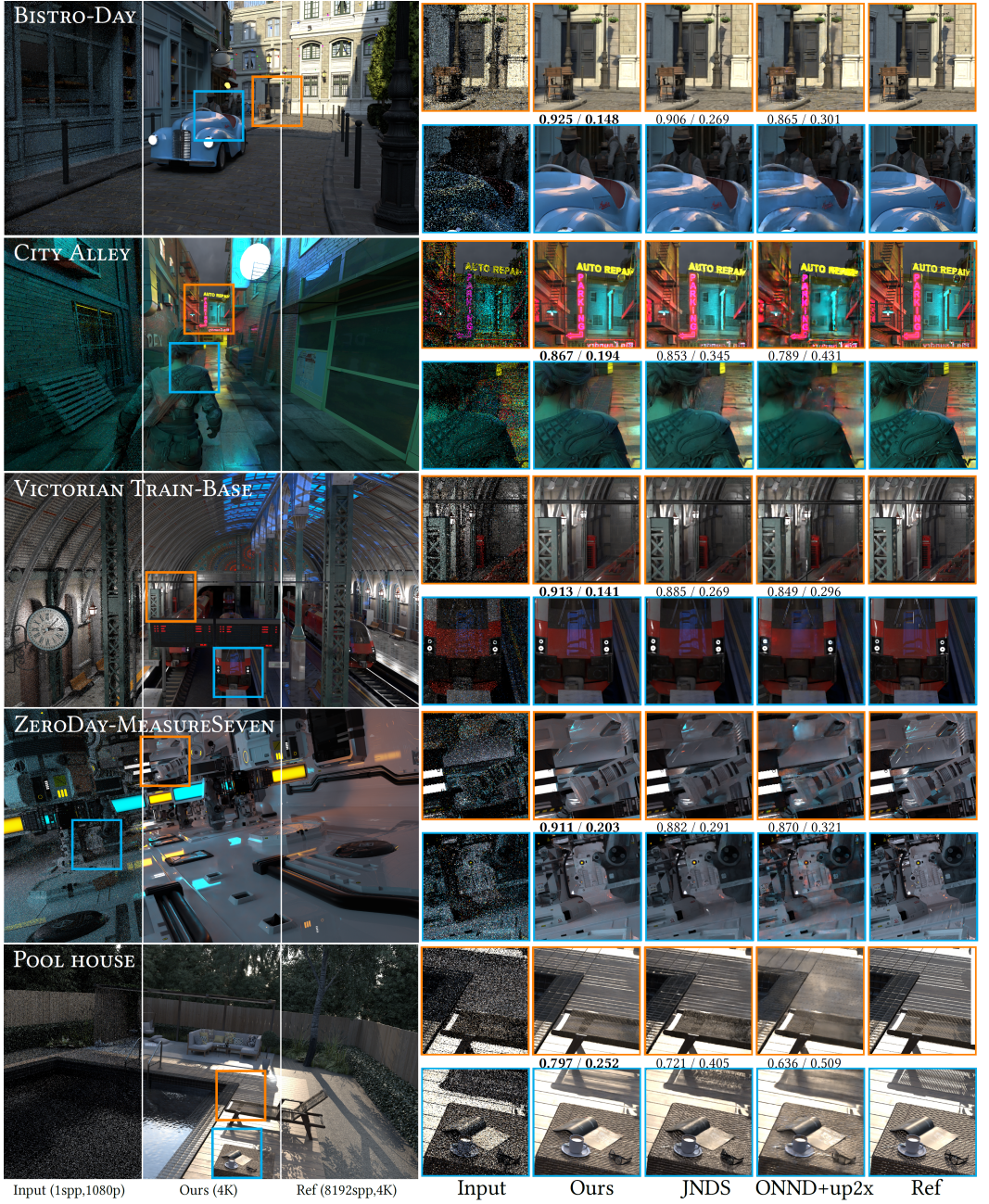
Fig. 4. Denoising and upscaling quality comparison from test dataset in 4K against prior works, JNDS [Thomas et al. 2022] and ONND [Nvidia 2021] with a built-in 2× upscale. Quality metrics (SSIM↑/LPIPS↓) are calculated on a full resolution image. We denote in bold the best quality score. Noisy input in 1080p is shown in 2× upscaled for visualization purpose. Our results outperform the prior techniques for these test dataset in visual and quantitative quality.
